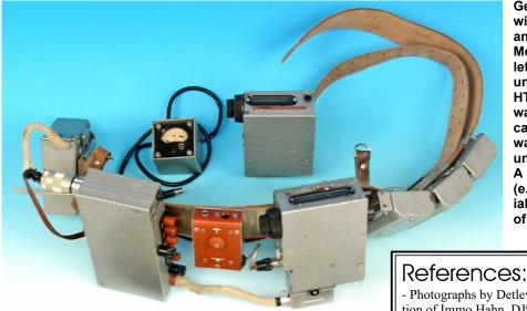
General view of 12026.1 (without wide band aerial) showing test meter and second RF unit on top.
